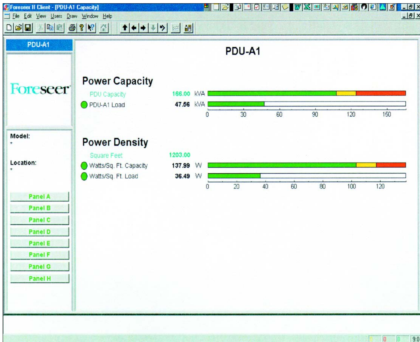
Figure 5. Power capacity vs. real-time load measurements per Power Distribution Unit. Calculation of watts per square foot for power density.
