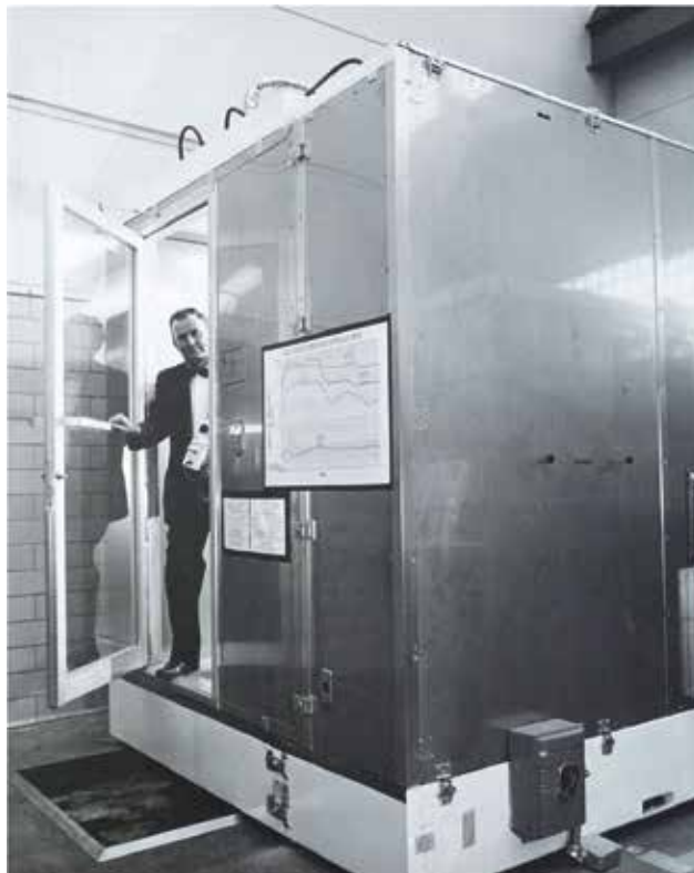
Willis Whitfield steps out of a mobile cleanroom, which could be transported to remote sites. Sandia National Laboratories
