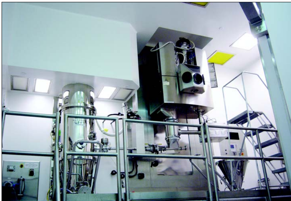
Integrated contained high shear granulator and fluid bed processor.
