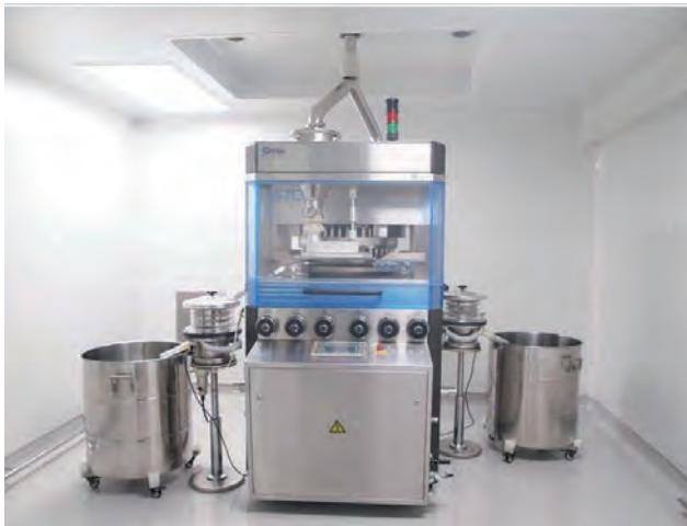
Tablet compressing set, granule transfer tube, tablet deduster and bulk product IBC
