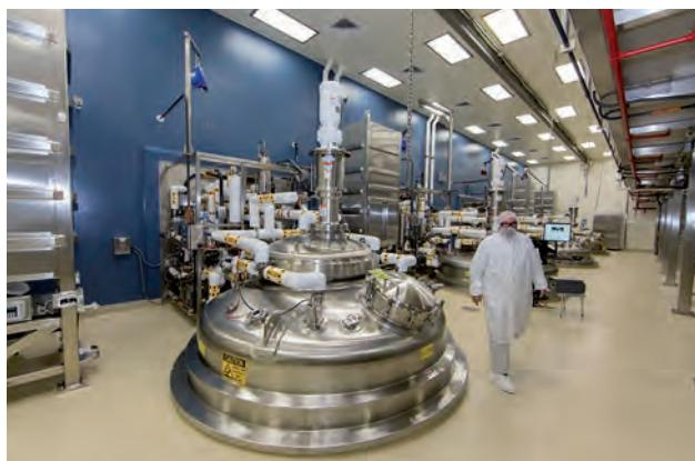
*This view shows the top-down flow of media prep area. The raw materials are added to the media prep tanks from above.*
