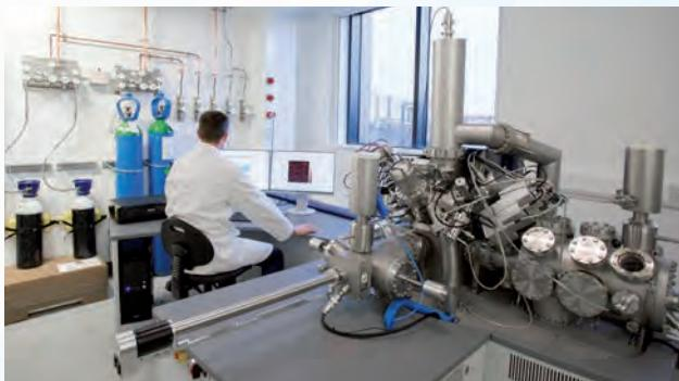
Time of flight secondary ion molecular spectroscopy instrument used for surface analysis
