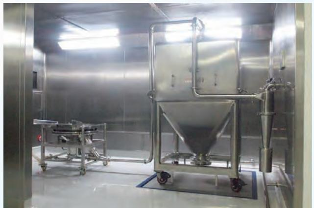
Raw material transferring into IBC with recovery cyclone in dispensing booth
